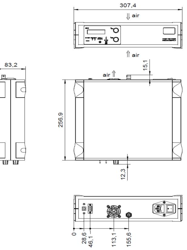
Figure 11: THQ Desktop, Example for 1 Channel up to 7kV
