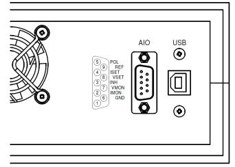
Figure 2: Example rear panel with AIO and USB
