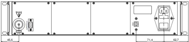
Figure 8: THQ 19 Zoll, Example for 1 Channel 30kV
