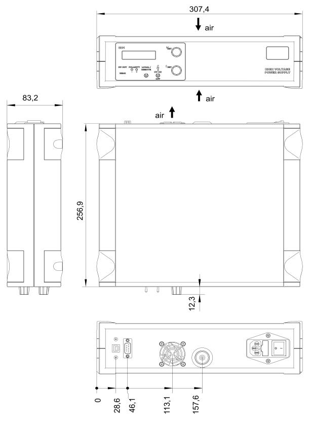
Figure 11: THQ DESKTOP, 1-channel 30kV (L30)
