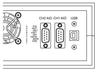
Figure 3: Rear panel with AIO and USB connectors
