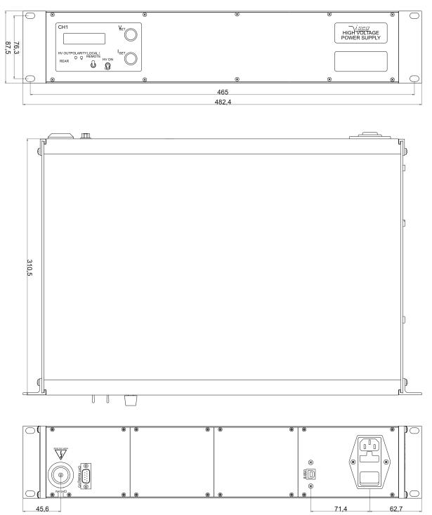
Figure 14: THQ 19-Zoll SYSTEM, 1-channel 30kV (L30)
