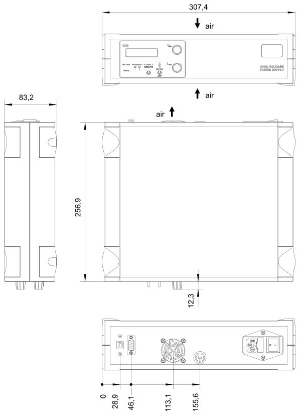
Figure 10: THQ DESKTOP, 1-channel 16kV (L16)
