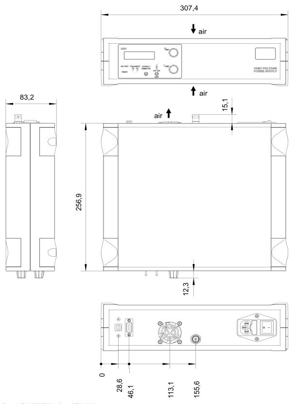
Figure 9: THQ DESKTOP, 1-channel 7kV (SHV)
