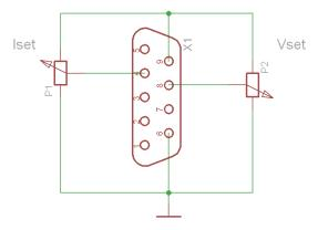
Figure 4: AIO circuit for simple V<sub>set</sub> and I<sub>set</sub> control
