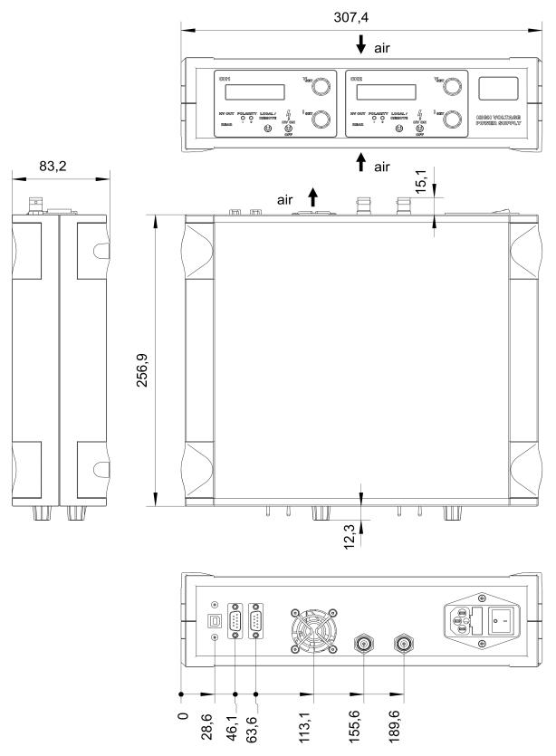
Figure 12: THQ DESKTOP, 2-channel 7kV (SHV)
