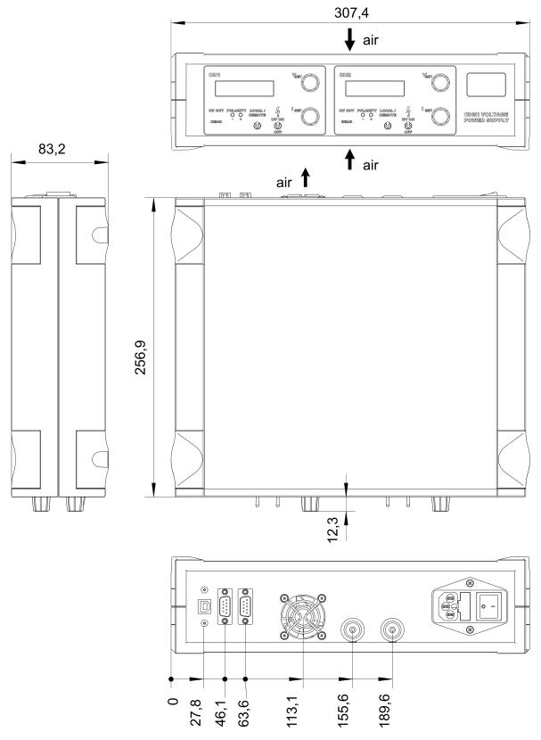
Figure 13: THQ DESKTOP, 2-channel 16kV (L16)
