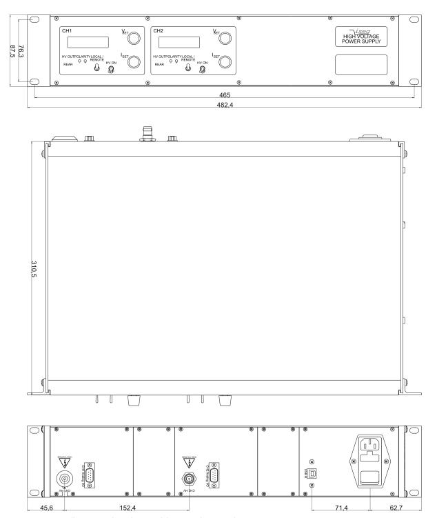
Figure 17: THQ 19-Zoll SYSTEM, 2-channel (EPS modules, L16 and SHV sample)
