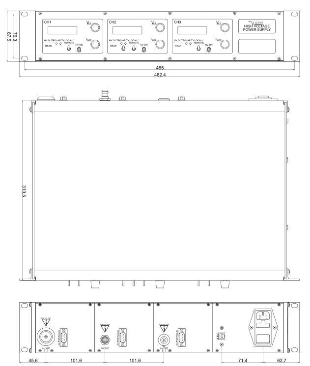
Figure 16: THQ 19-Zoll SYSTEM, 3-channel (L30, SHV and L16 sample)
