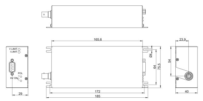
Figure 10: dimensional drawing DPS with SHV
