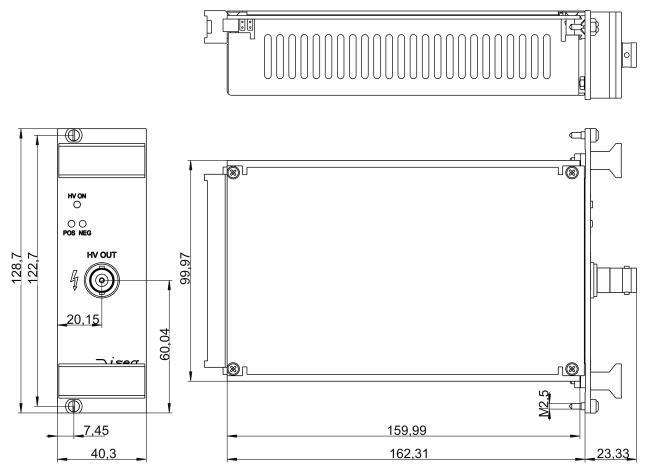
Figure 11: dimensional drawing DPS 3UC
