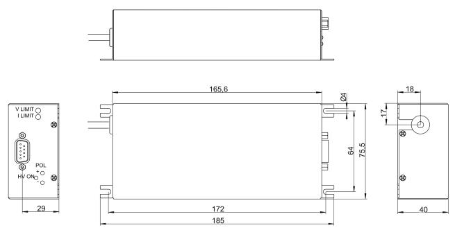
Figure 9: dimensional drawing DPS with cable
