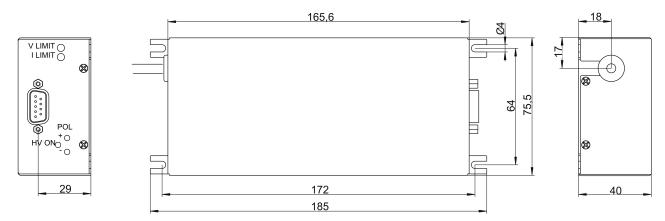
Figure 9: dimensional drawing DPS with cable
