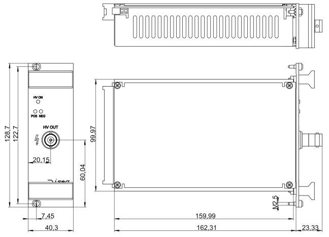
Figure 11: dimensional drawing DPS 3UC
