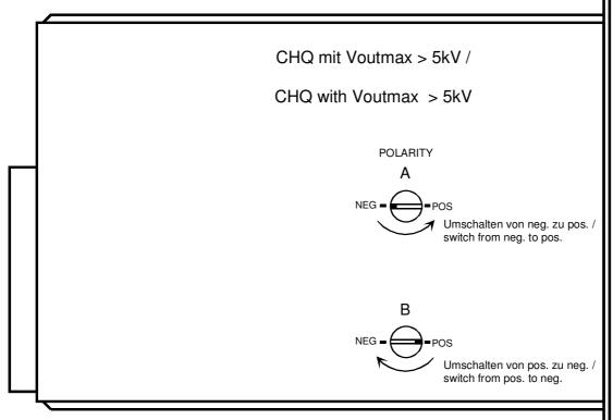
**Appendix B:** CHQ side coffer, Polarity rotary switch
