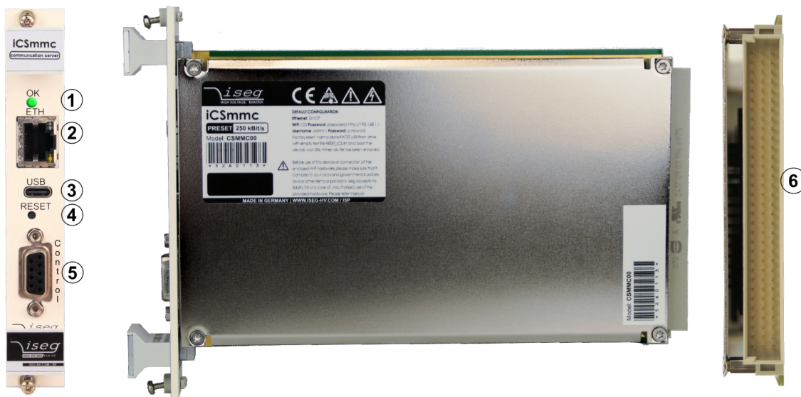
Figure 1: Sample of MCC controller
