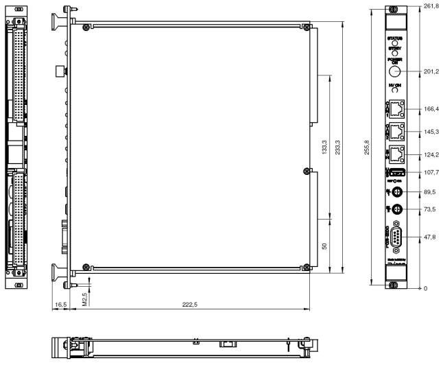
Figure 14: Dimensional drawing CC24, MASTER
