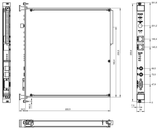
Figure 13: Dimensional drawing CC23, SLAVE
