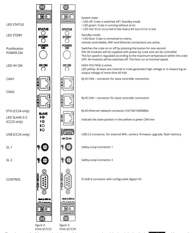
The voltage supply of the crates backplane and the crate connected modules is switched on by the POWER ON pushbutton or by remote control.
