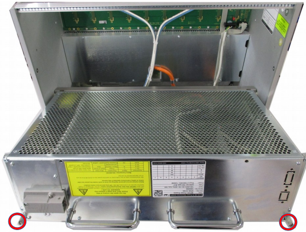
Figure 3: remove wire tie and loosen screws
