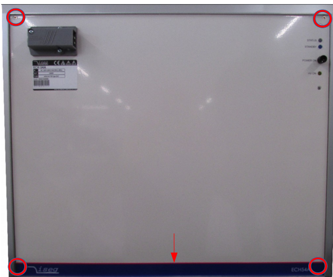
Figure 1: remove blue sticker , undo 4 screws
