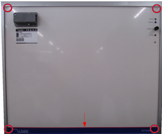
Figure 1: remove blue sticker, undo 4 screws
