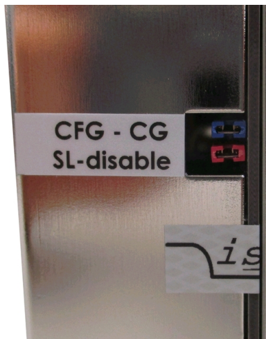
Figure 1: Jumper configuration on back side
