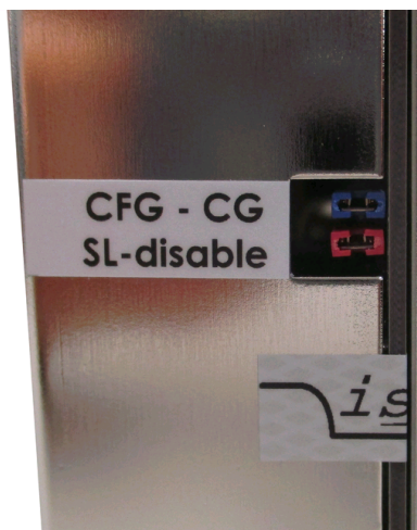
Figure 1: Jumper configuration on back side
