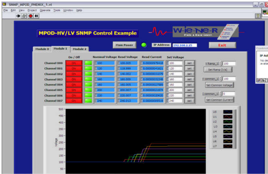
Example for LabView VI for 8 channel high voltage module
