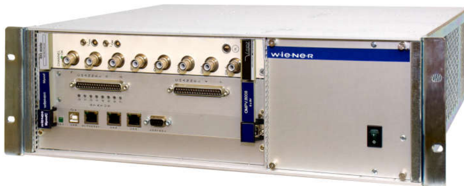
MPOD micro_2 crate with MPOD controller, one low voltage and one high voltage module
