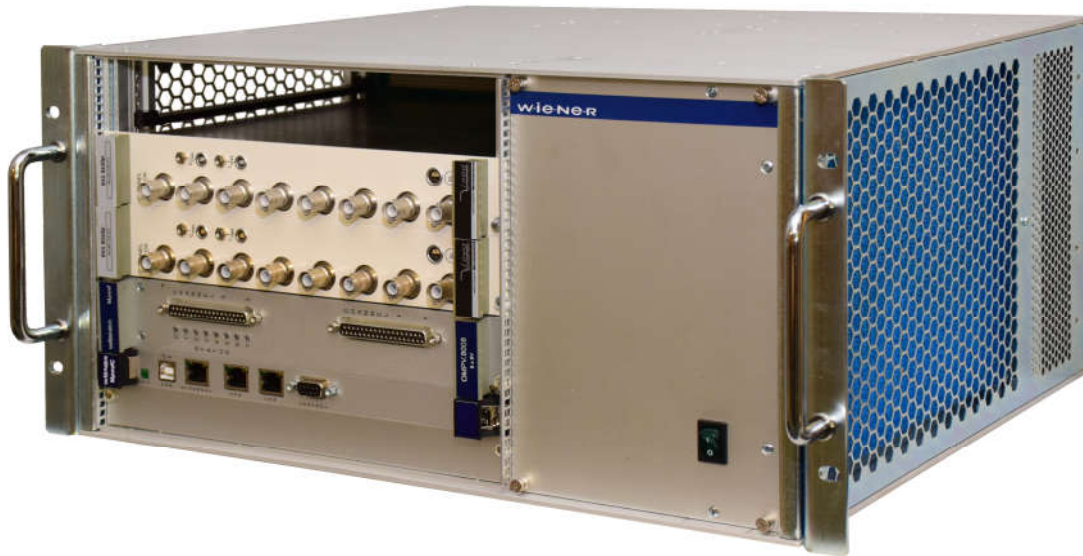
MPOD Mini crate with MPOD controller and 2 high voltage + 1 low voltage module
