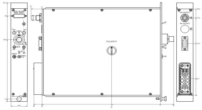
Figure 4: Dimensional drawing - NHQ 1 channel
