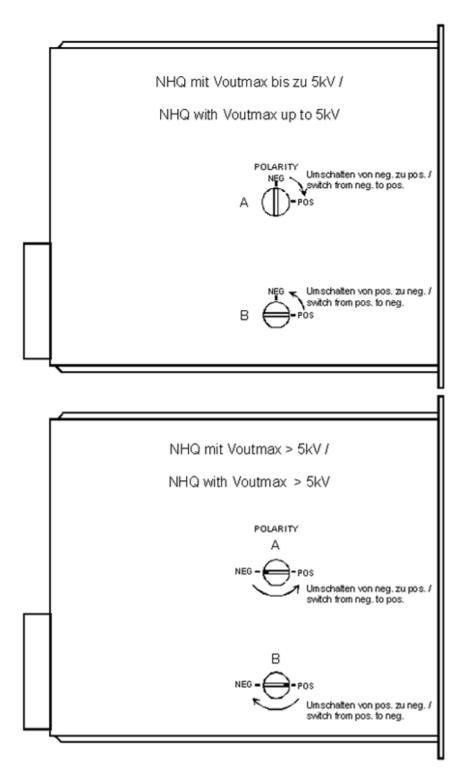
Figure 3: Polarity Switch – Side view
