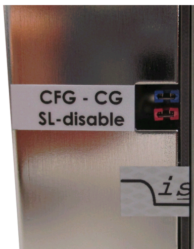
Figure 1: Jumper configuration on back side
