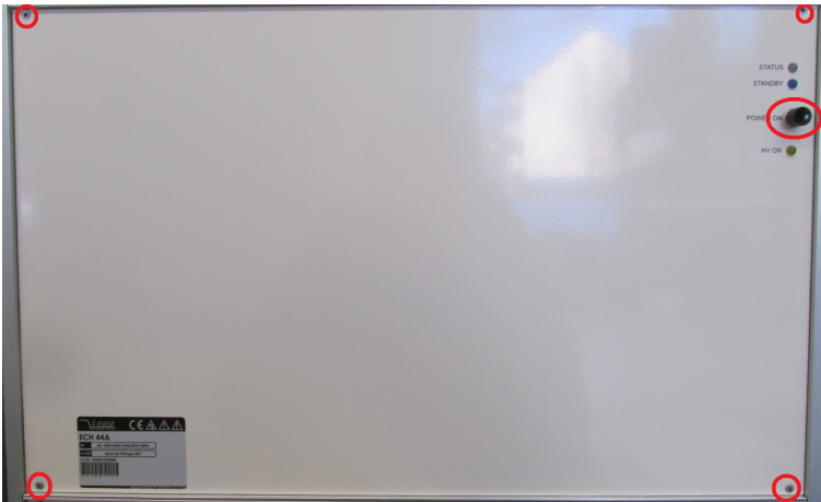
Figure 1: Remove back cover to replace power supply
