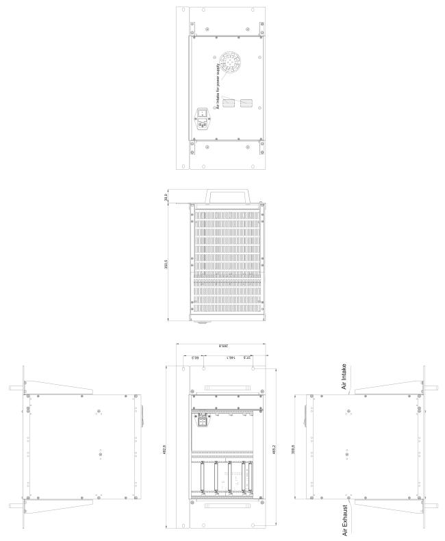
Figure 4: Dimensional drawing ECH 244 with Option RAC
