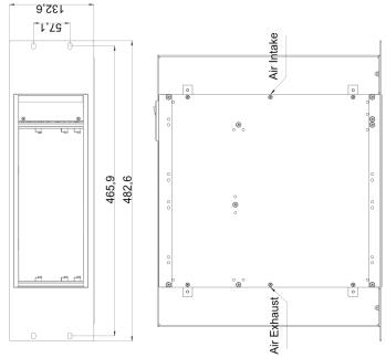
Figure 2: Dimensional drawing ECH 242 with Option RAC
