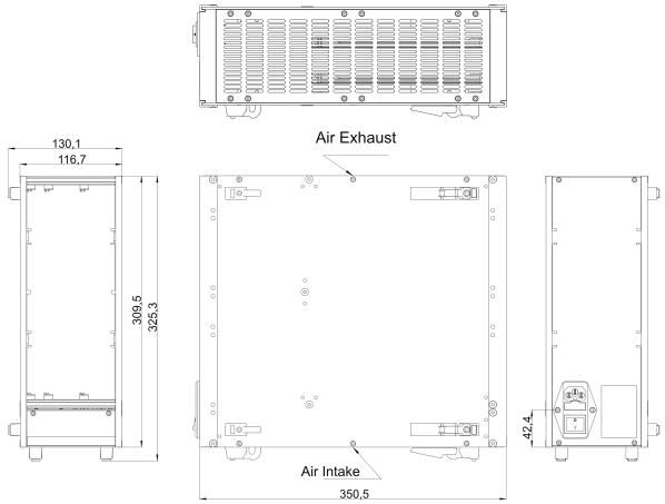
Figure 1: Dimensional drawing ECH 242 – 2 channel MMS crate
