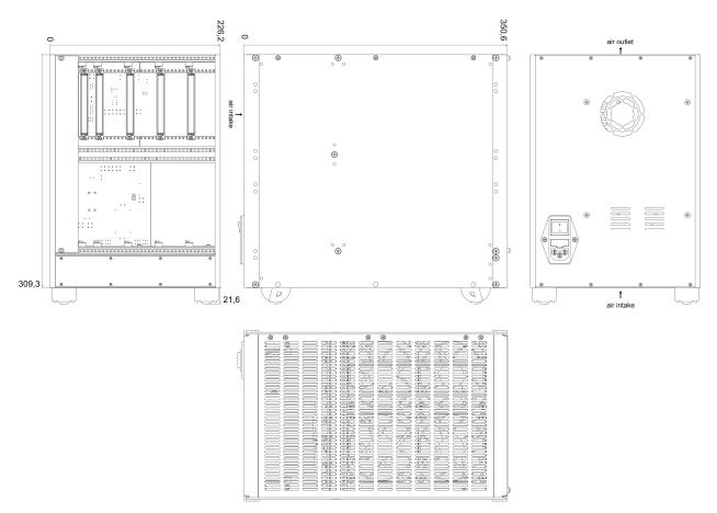
Figure 3: Dimensional drawing ECH 244 - 4 channel MMS HV crate
